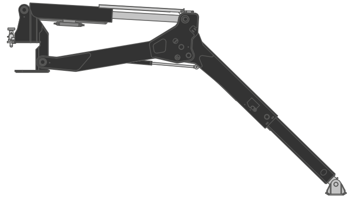
45° EXTENSION WITH OUTRIGGER COMPLETELY UNTHREADED
