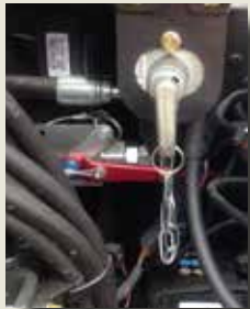
Battery kill switch for storage and theft protection
