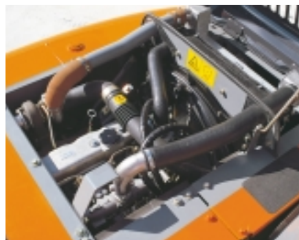
A low-noise muffler and the Isuzu Tier 2 emissions control engine ensure a quieter, more environmentally friendly excavator. Plastic parts are labeled for easy recycling. Wiring is lead-free.
